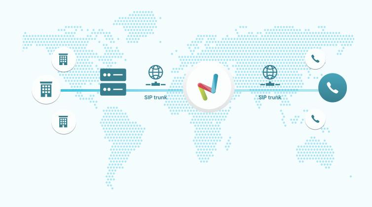
SIP trunks can act as a bridge between a traditional phone line (PSTN) and VoIP. They help you easily set up voice connections with VoIP and route calls across the globe. Both inbound and outbound.
